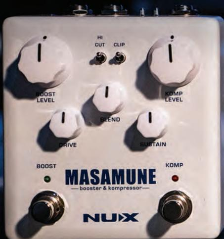
Analog compressor and booster pedal
