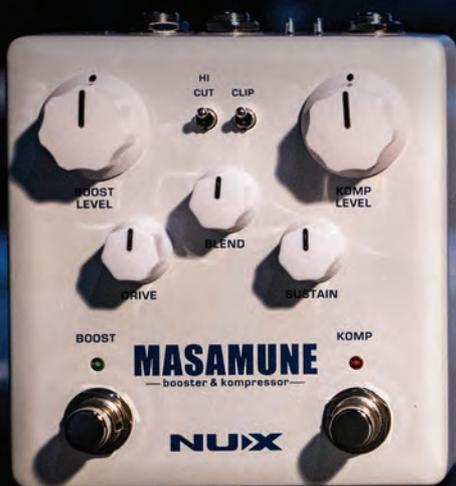
Analog compressor and booster pedal
