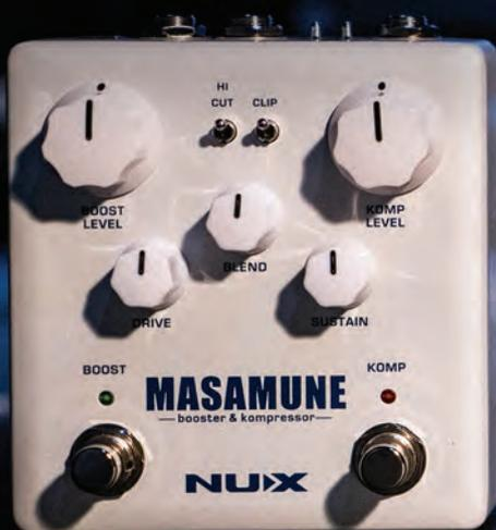
Analog compressor and booster pedal
